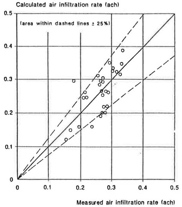
Fig. 2. Comparison between calculated and measured air infiltration rates (HUDAC standard house).
