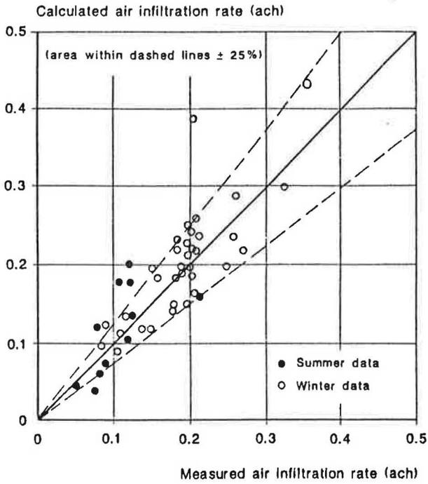
Fig. 1. Comparison between calculated and measured air infiltration rates (HUDAC upgraded house).
